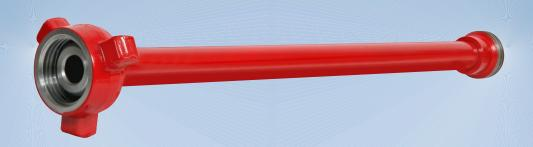
Shreeraj Industries offers NPST (Non-pressure Seal Thread) Pups in size 1"-3" Fig 602 and 1502. The NPST connection offers a light weight pup capable of 6000 15000 CWP with a connection that isolates the thread from fluid's flowpath. This connection is permanent and is well suited to abrasive applications where a welded connection is not desirable.
